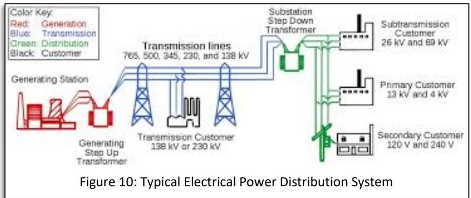
Figure 10: Typical Electrical Power Distribution System
